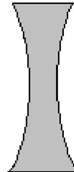
In a diverging lens, the waves slow down more at the lens' edges, (thinner in the middle), and the light diverges.
